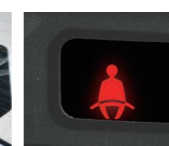
The system sets off a sound alarm with a light lit to warn that the seat belt is unfastened.
